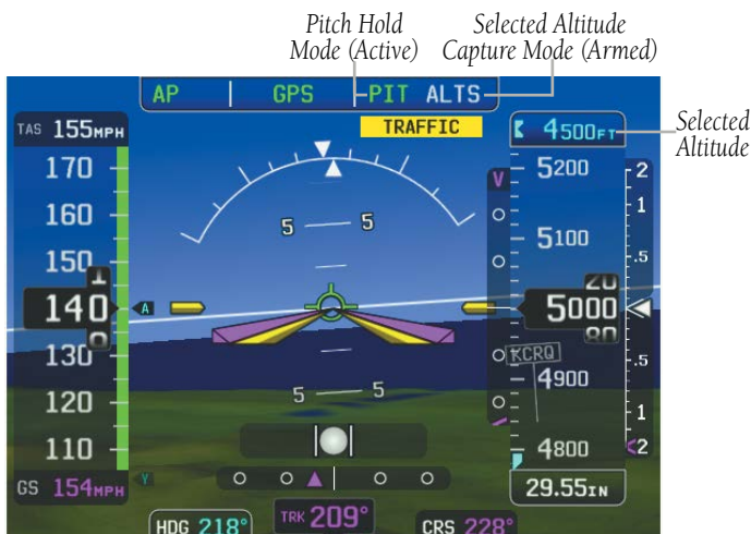
Pitch Hold & Selected Altitude Capture Modes
