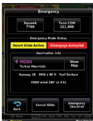
Prompt to Disengage Autopilot (Emergency Page)
