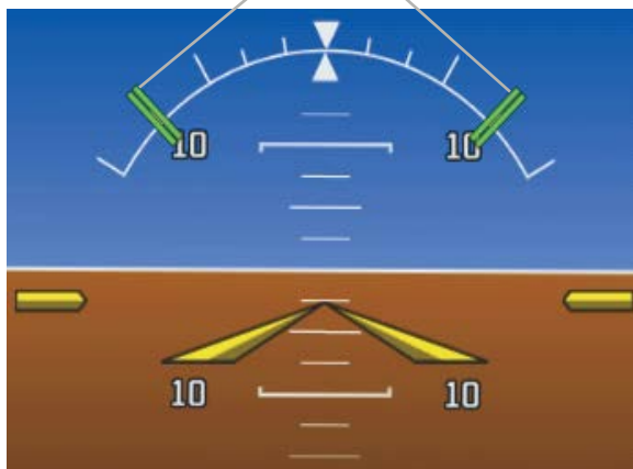
ESP Roll Engagement Indication (ESP Enabled but NOT Engaged)
