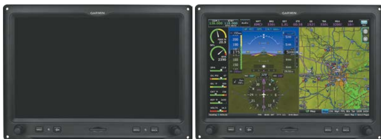
G3X Touch Full-Screen Reversionary Mode (Failed PFD)
