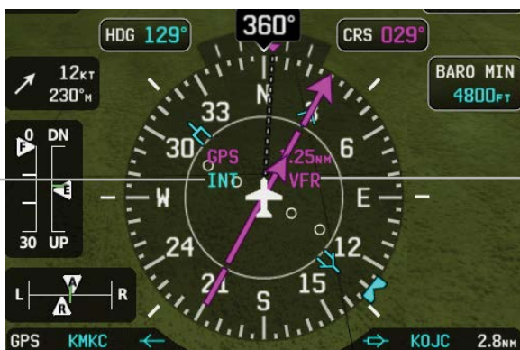
Intentional Pilot Selection of Internal GPS Navigation
