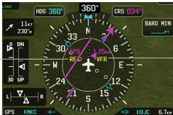
External GPS Navigator Failure
